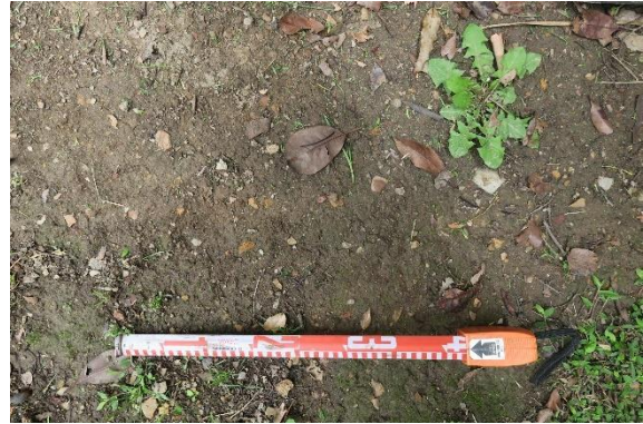
Figure 23. Exposed soil on the northern side of 683-685 Old Northern Road. Soil is mixed clay with gravel and brick fragment inclusions.
