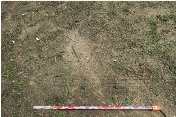
Figure 24. Exposed soil on the western side of 683-685 Old Northern Road, on the slope between the house and Old Northern Road. Soil is a mixed loamy sand with some gravel inclusions.
